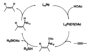
Pd(0) - acetic acid catalyst system suggested such a process might be intrinsically more chemoselective compared to heterogeneous catalysts.
